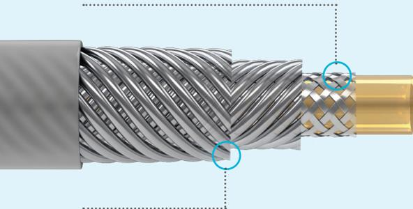
Dual-layer, bi-directional coils expand and collapse depending on the orientation of rotation, working together to create a gear-like mechanism to transmit torque from hub-to-tip
